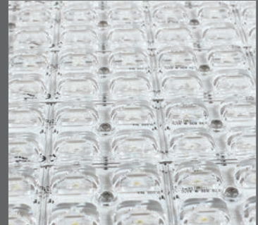
Each Led is associated with a specific lens that generates the photometric distribution of the light.
