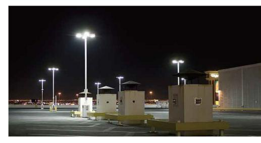
The luminiare has multiple roadway lighting distributrions designed to maximized spacing while meeting stringent requirements of IES RP8 guidelines for average, uniformlity and veiling luminance. Installation costs are minimized with this direct retrofit luminaire without rewiring or changing existing luminaire arms. Asymmetric distributions are easily aimed towards the roadway with the rotable optical assembly.
